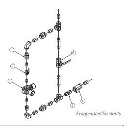
SERIES 757P AIR MAINTENANCE TRIM ASSEMBLY WITH PRESSURE SWITCH
