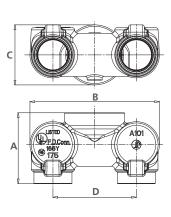
► Concealed auxiliary inlet with 500 G.P.M. inlet capacity to supplement Fire Protection water supply.
