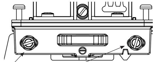
Slotted mounting holes and micro-adjustment feature may be used for fine adjustment of switch assembly to mounting bracket. Re-tighten screws to 20 in-lbs minimum.
