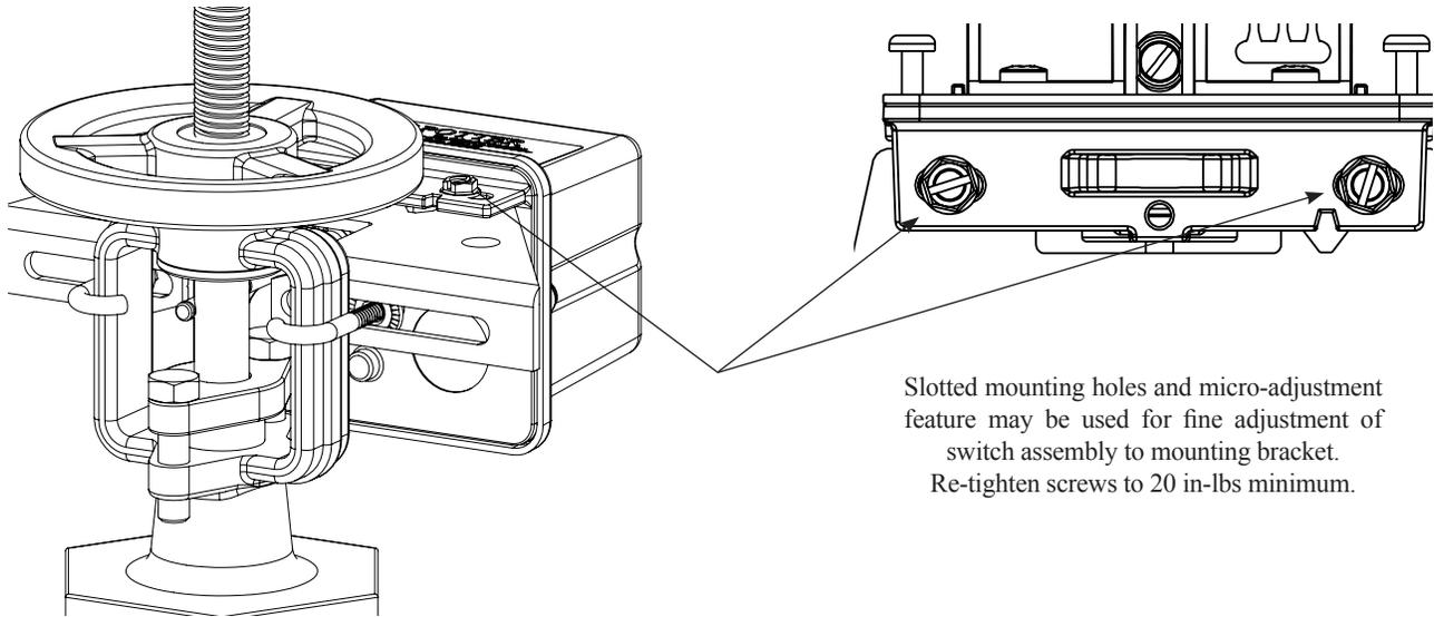
Slotted mounting holes and micro-adjustment feature may be used for fine adjustment of switch assembly to mounting bracket.
