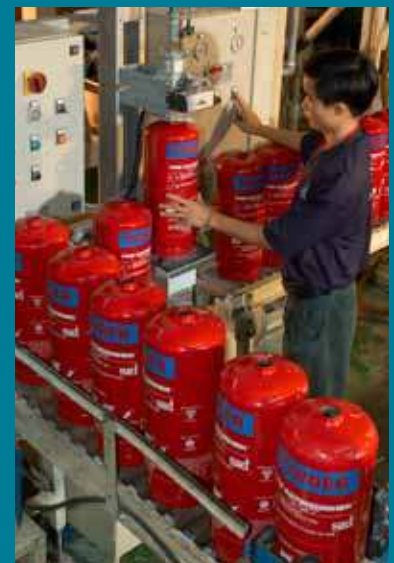
▲ Fire Extinguisher Powder Filling
