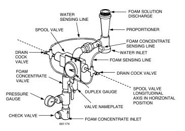
**Note:** Spool valve must be installed with the longitudinal axis in the horizontal (level) position.
