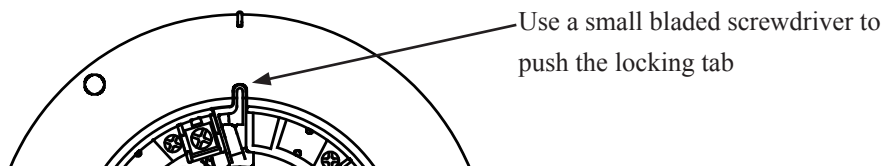
Figure 2. Removing of detector head from base
