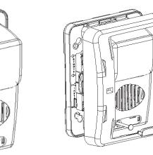
To remove bezel, grip both sides of bezel and pull in a download and outward motion.
